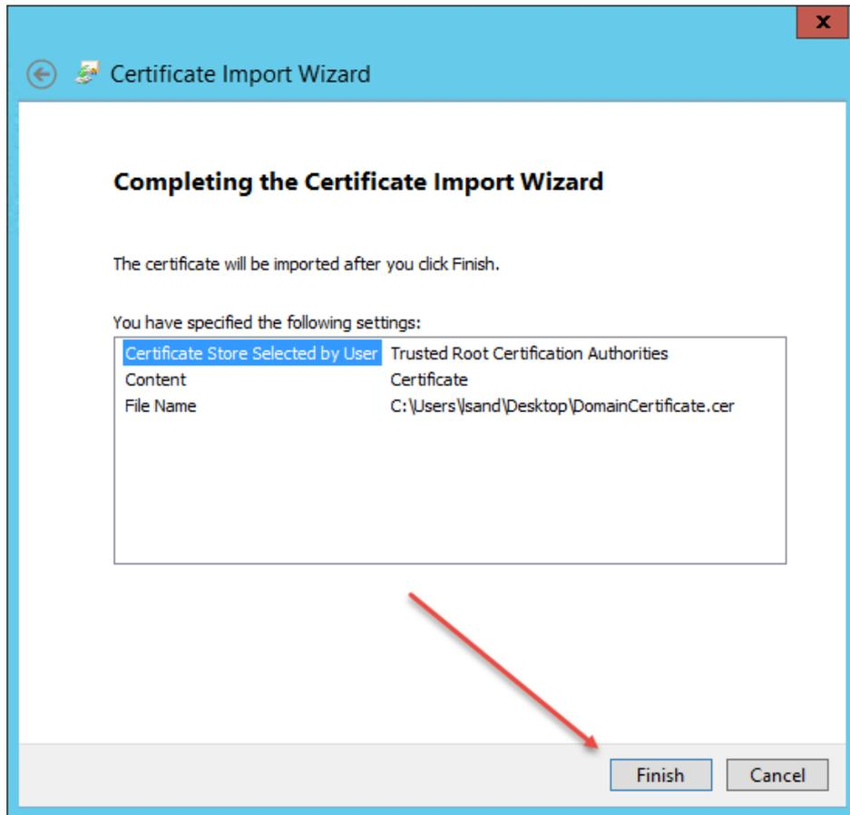
8. This ends the import process, and your domains should now be able to securely communicate using **LDAP over SSL**
